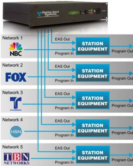
One DASDEC-II MultiStation provides complete simultaneous EAS coverage for up to 5 networks.
