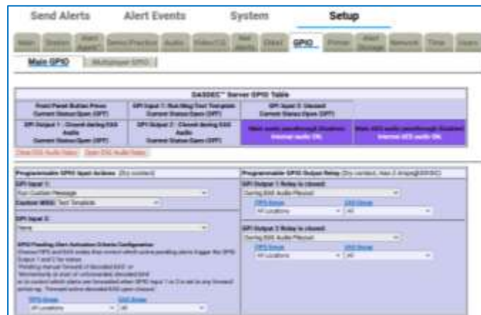
Main GPIO - GPI Setup Screen
