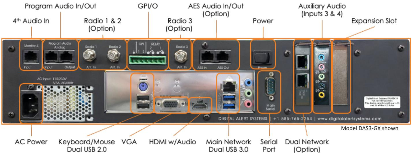
Besides offering AES as a module, the DASDEC-III introduces RJ-45 style audio connectors replacing bulking and expensive XLRs or difficult to patch terminal strips. The new audio connectors allow simple CAT5/6 wiring with many of the latest audio consoles and devices, following a standard wiring configuration so customers can purchase any number of adaptors (available separately) or craft their own.
