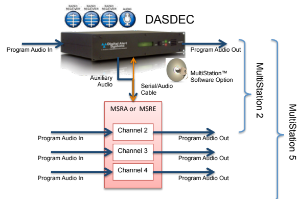
Figure 1 DASDEC and MSRA configured for 4 discrete program streams (requires MultiStation-5 for more than two channels).
